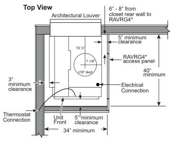
For RAVRG4\*: After installing RAVDPLAT per instructions, slide rear of unit through RAVRG4\* and rest it on platform in the closet. Rotate unit 90° so that rear of unit is facing the wall plenum. Follow remaining instructions for installing unit to wall plenum.
