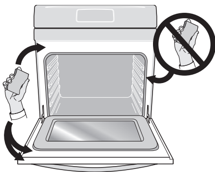
Figure 16: Clean around the oven door gasket
