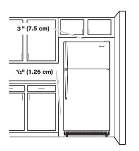
To ensure proper ventilation for your refrigerator, allow for a  $\frac{1}{2}$ " (1.25 cm) space on each side. Allow 3" (7.5 cm) of space between overhead cabinets and refrigerator top. Allow at least 1" (25.40 mm) between back of cabinet and the wall. If your refrigerator has an ice maker, make sure you leave some extra space at the back for the water line connections.
